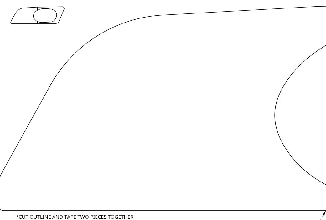
\*CUT OUTLINE AND TAPE TWO PIECES TOGETHER AT "CUT LINE". FLIP TEMPLATE OVER FOR PASSENGER SIDE.
